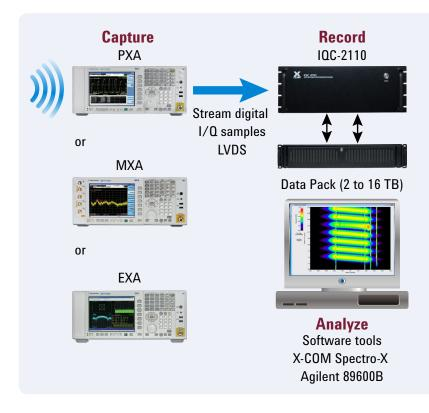
capture time is possible at a 10 MHz bandwidth and over 15 hours at the full 40 MHz capture bandwidth. Captured files can be transferred to an X-COM SigAnalyst workstation with a comparable amount of RAID5 disk storage for post processing.
